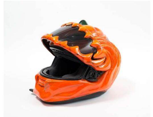
This was a 3D scan project, starting with a 3D scan of a base helmet (Shoei off-shelf performance helmet) and then scanning a clay sculpt on top of the base helmet, and digitally subtracting the difference to re-create the parts for subsequent assembly via 3D printing.
